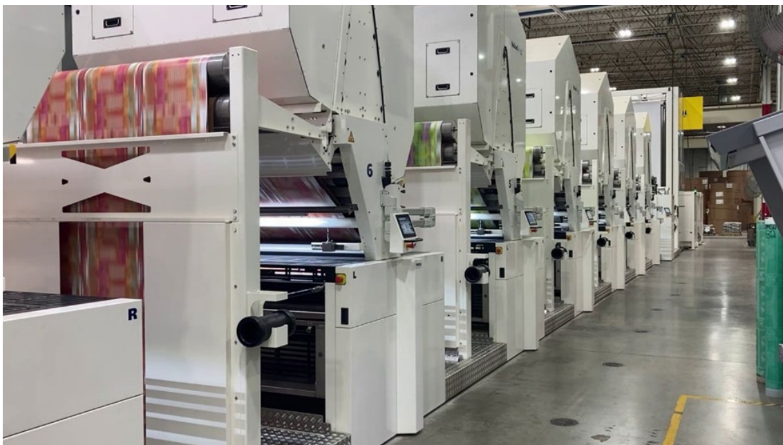
The new Next Generation TRESU Flexo Innovator's modular design supports single or dual ink-deck configurations, giving converters flexibility for diverse job mixes and job changes on the fly — with minimum waste.
