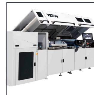
Inline or stand-alone coaters or units TRESU iCoat II: Up to 4,600 sheets/hr
