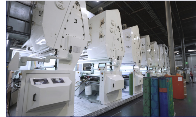
Largest installed base of inline flexo printing units world-wide. TRESU Flexo Innovator: 67” and 2,600 ft/min (800 m/min)
