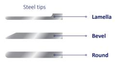
**Lamella** Lamella profiles are used in coating but also gravure and flexo printing. A lamella profile wipes well, up to the point that the contact zone becomes too large. They are available in different angles- pls. inquire for more details.
