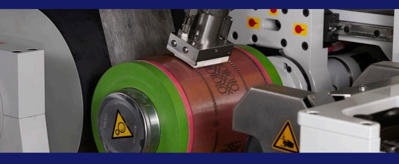
More uptime with automated inline cleaning of print plates for tissue or napkin production: No physical contact, no handling, maximum safety.
