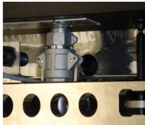
Photo showing "foam-free" coating draining out of the chamber and into the overflow pan
